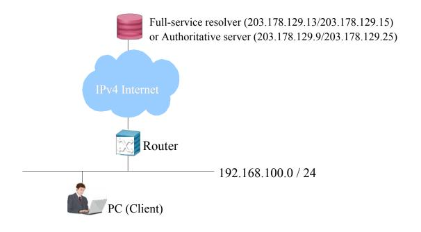
\* CentOS5.4 is used for PC (Client). BIND-9.7.0rc1 is installed.
