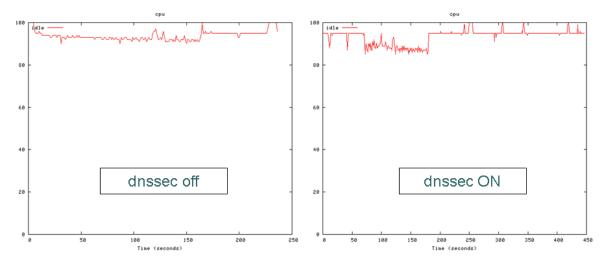
It was verified that the CPU load increased when DNSSEC was on compared to when DNSSEC was off. (Due to the band width restrictions of the upper network, the processing number of DNS decreased and the full CPU capability could not be utilized.)
