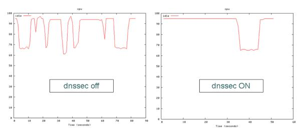
The CPU load with the cache hit rate of 100% showed the same value when DNSSEC was on and when DNSSEC was off.
