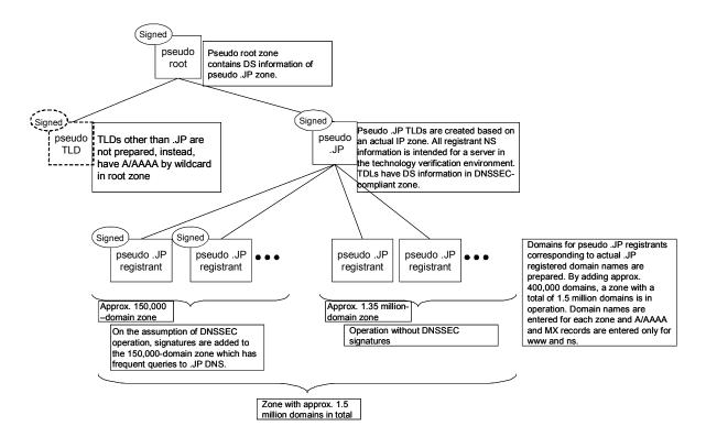
In order to make a comparison of the environment with and without DNSSEC, JPRS also created a pseudo tree without a domain name signature in a .JP zone (the same as an ordinary DNS tree), which is not shown in the above diagram. In addition, JPRS set up a cache DNS server linked to the pseudo DNS tree.
